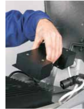
Removing the driver
