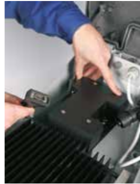
Mounting nuts unscrewing of the driver and disconnecting the power plug without any tools
